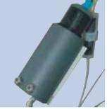
A galvanic cell oxygen electrode determines Dissolved Oxygen. A semi-permeable membrane allows oxygen molecules to pass into the internal electrolyte; reduction at the gold cathode produces a voltage output that is temperature compensated and proportional to oxygen concentration.
