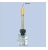
An ammonia gas electrode is modulated in a special flow cell.
